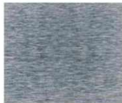
Surface finish: fine-machined, and grinded, Ra 0.2 μm
