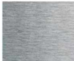
Surface finish: machined, Ra 0.8 μm
