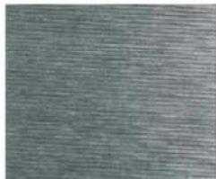
Surface finish: machined, Ra 1.2 μm
