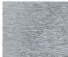
Surface finish: fine-machined, and grinded, Ra 0.4 μm
